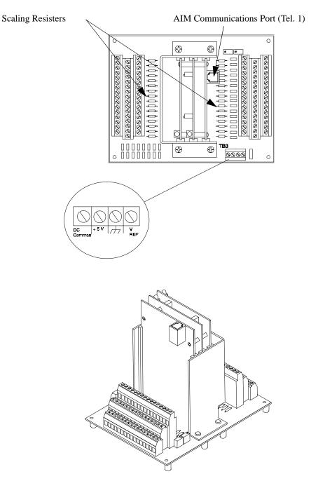
This figure shows the AIM cards (also known as the MUX cards) and AIM-TB, with scaling resistor locations.
