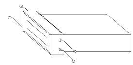
3. Remove the electronics assembly from the case, as shown below.
