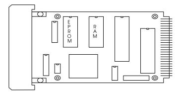
6. Remove the existing EPROM from its socket by prying it out with a small flathead screwdriver, as shown below.
