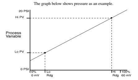
Before you enter the values that determine the two points for the conversion line, you must choose an appropriate display format. The MLS has six characters available for process variable display; select the setting with the desired number of decimal places before and after the decimal point. Use a display format that matches the range and resolution of the process variable. The display format you choose is used for the setpoint, alarms, deadband, spread, and proportional band.
