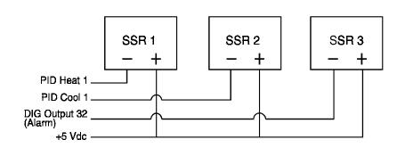
System Safe (Watchdog Timer) constantly monitors the MLS CPU. It is a SINK output located on RTB terminal #6. (Do not exceed the 10 mAdc rating for the System Safe output.) Its output is Low (on) when the CPU is operating; when it stops operating, the output goes High (off), de-energizing the SSR.
