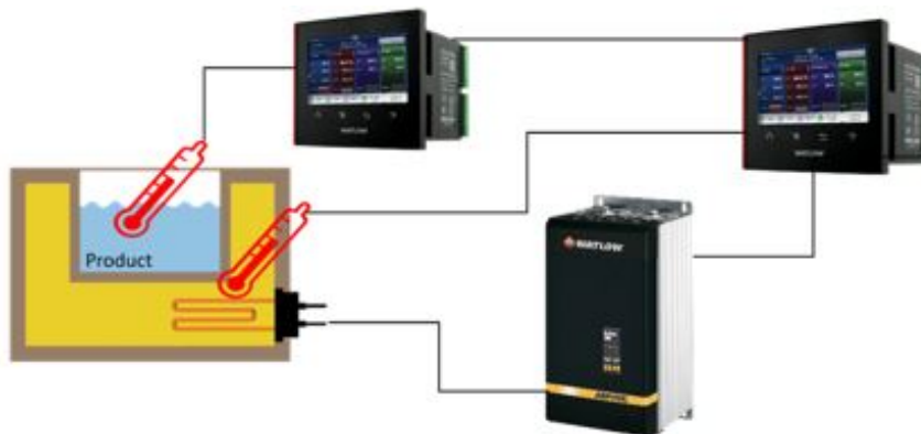
Figure 2 – Cascade control system
