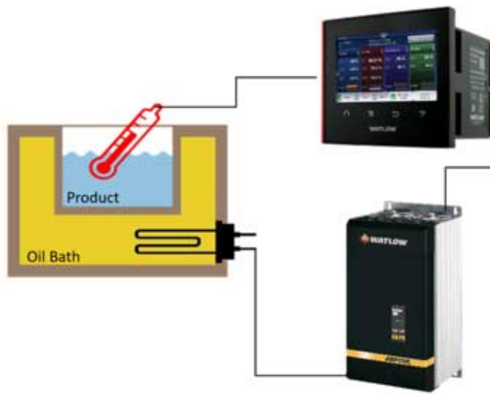
Figure 1 – Single loop control system
