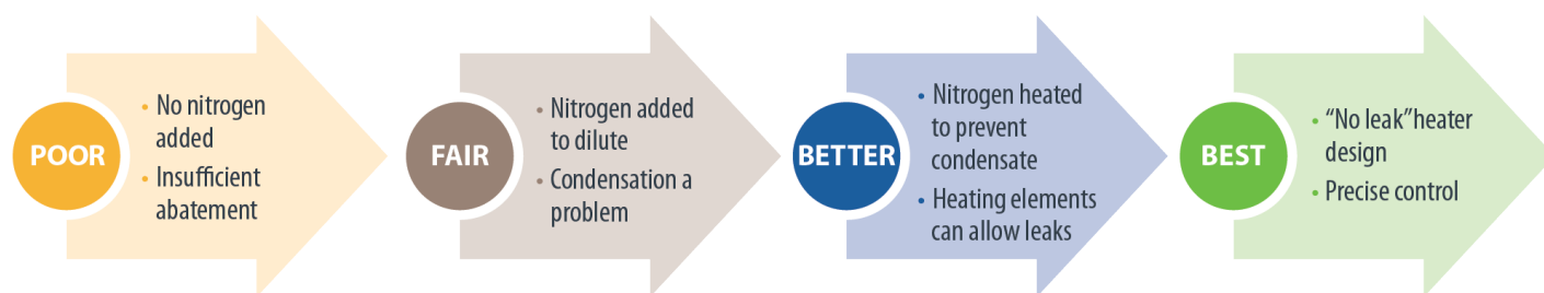
Figure 2: Stages in the problem-solution space of semi-fab exhaust abatement
