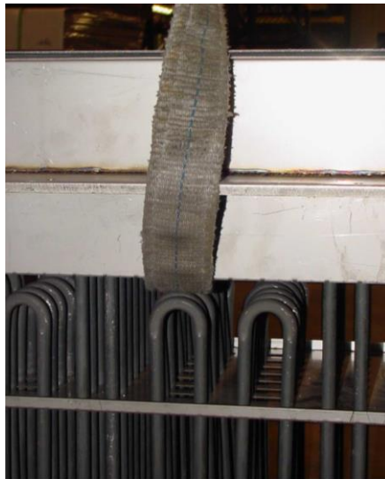
Figure 4 - For Vertical lifting place strap through the space between the element bundle and the insulation retainer. Do not slip the strap through the elements.
