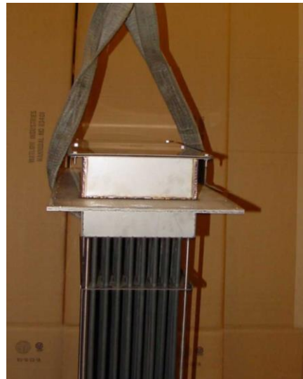
Figure 4 - For Vertical lifting place strap through the space between the element bundle and the insulation retainer. Do not slip the strap through the elements.
