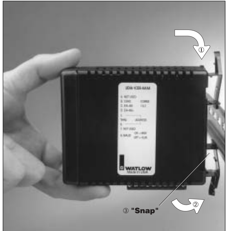
Figure 10a - Mounting a MicroDIN controller on a DIN rail
