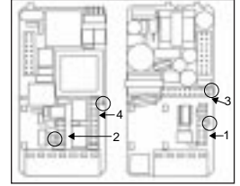
Figure 3 — Main boards and numbered output slots
