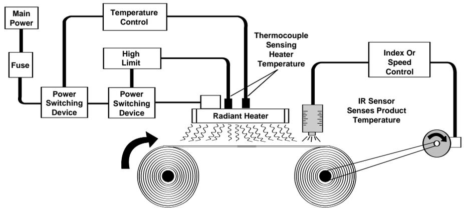
**Product Temperature Sensed and Used to Control Product Speed.
