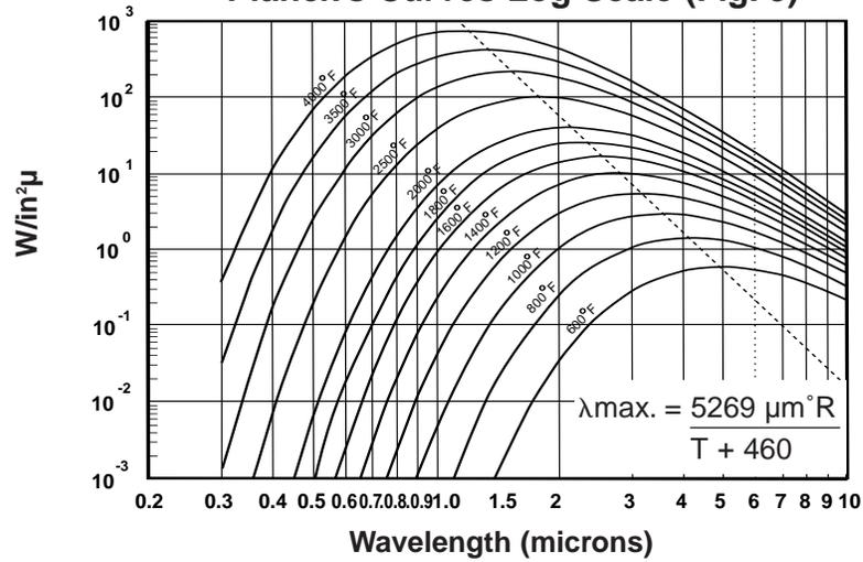
Blackbody Radiation By Micron Band Widths (Fig. 4)
