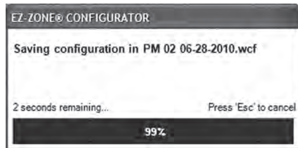
Saves complete sets of parameter settings for backup, archiving or configuring other devices with the same settings.
